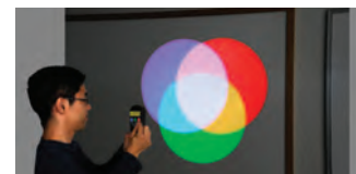
Use as a projector in classroom demonstrations. Individually adjust the intensity of the super bright red, green, and blue LEDs.
