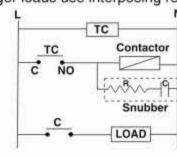
NOTE: Use snubber as shown above to increase life of internal relay of temperature controller.
