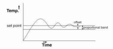
3) Offset adjustment (manual reset): After some time the process temperature settles at some point and there is a difference between the set temperature & the controlled temperature. This difference can be removed by setting the manual reset value equal & opposite to the offset.
